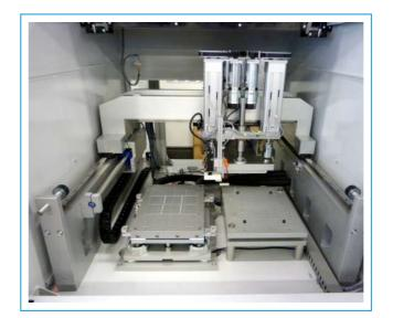
PV <u>Assembly</u>. DSSC glasses alignment and curing. Top & bottom vision alignment.
