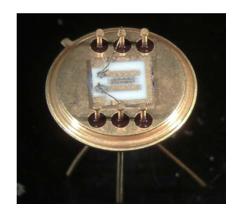
Sensor working by single sensitive lines printed by ink jet
