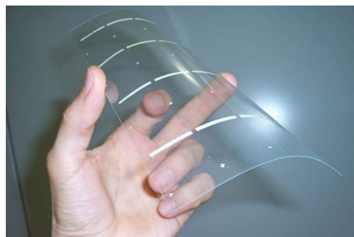
Ag based conductive ink on polymeric film for metamaterials production
