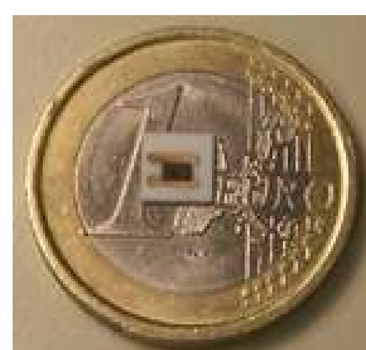
Sensor completely made by ink jet printing technique
