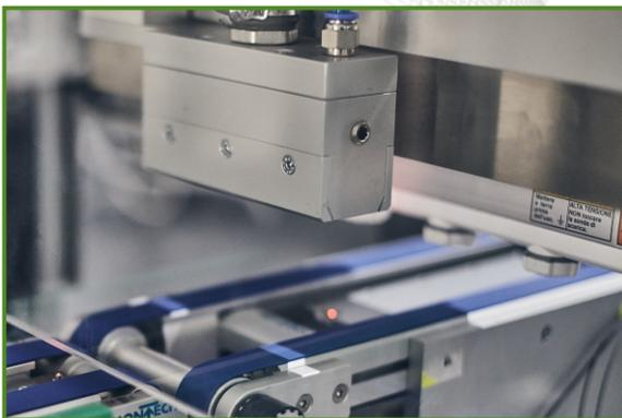
**CLEANING STATION WITH AIR KNIFE & IONIZER BAR**
