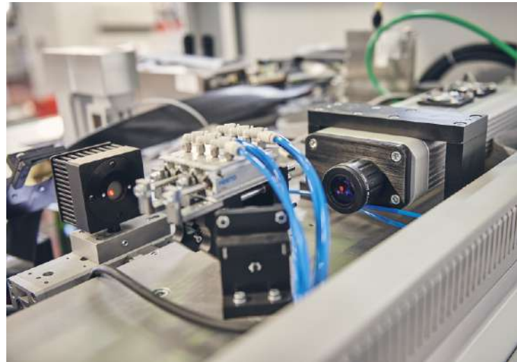
DIODE PUMPED GENERATOR INFRARED (1064 nm) or GREEN (532 nm)
