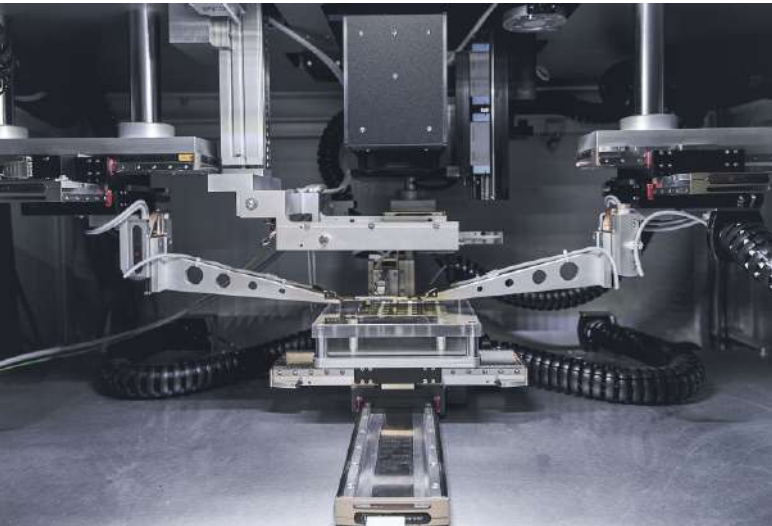
EXAMPLE OF PROBING SYSTEM WITH 3 FLYING PROBES (WITH ACTIVE PIN GUARD MODE)
