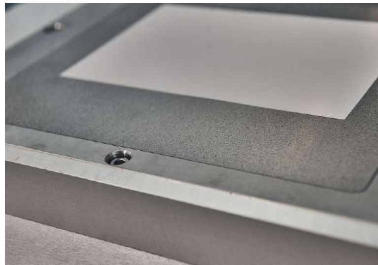
POROUS TABLE FOR FLEXIBLE SUBSTRATES & GREEN TAPE
