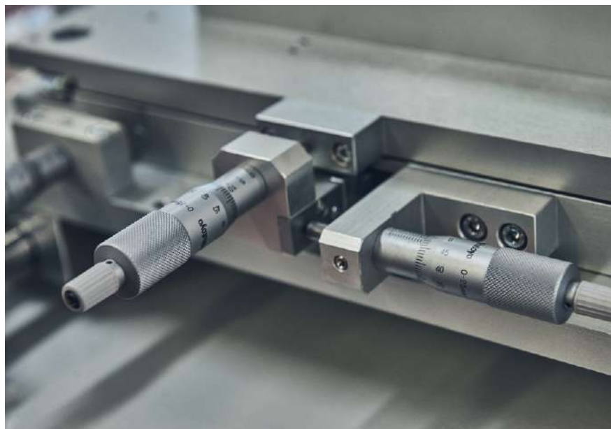
WORK-TABLE MANUAL ALIGNMENT BY MICROMETERS
