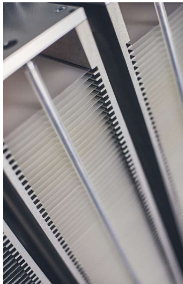
CASSETTE MAGAZINE FOR CERAMIC SUBSTRATES
