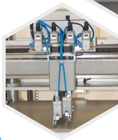
DOUBLE SQUEEGEES HEAD PRESSURE CONTROL BY SW
