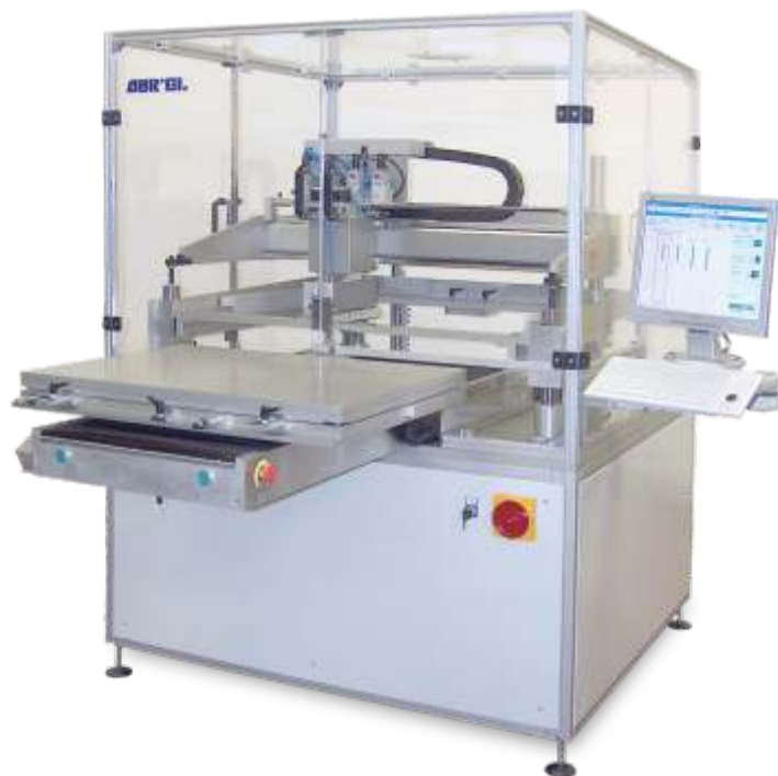
DOUBLE SQUEEGEES HEAD PRESSURE CONTROL BY SW
