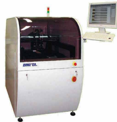
XCEL machine for microspray, dispensing, vision system, assembly.
